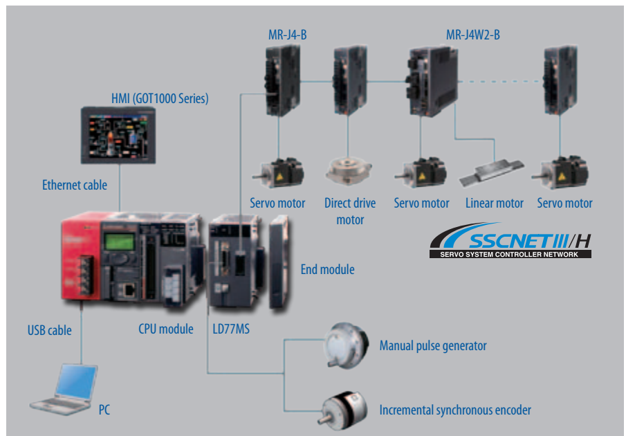
Structure of a system configuration comprising servo amplifiers and servo motors together with an MELSEC L Series PLC-CPU.
